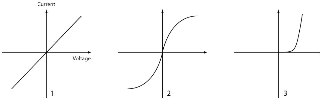
Figure 1: I-V characteristics for three different circuit components.
