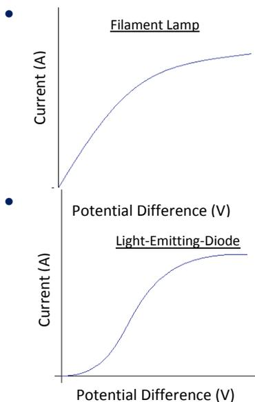
This is known as non ohmic; the current is not proportional to the potential difference. This is because the temperature changes as increased current passes through the filament. It is ohmic for small potential differences
