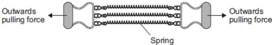
A person pulls outwards on the handles and does work to stretch the springs.
