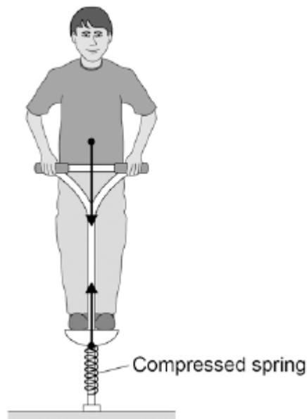
(a) The downward force of the child on the spring is equal to the upward force of the spring on the child.
