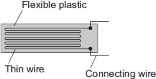
(a) (i) Using the correct symbols, **add** to the diagram to show how a battery, an ammeter and a voltmeter can be used to find the resistance of the strain gauge drawn above.
