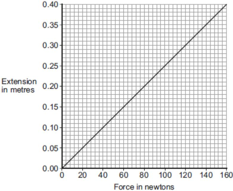
(i) How can you tell, from Figure 2, that the limit of proportionality of the spring has not been exceeded?
