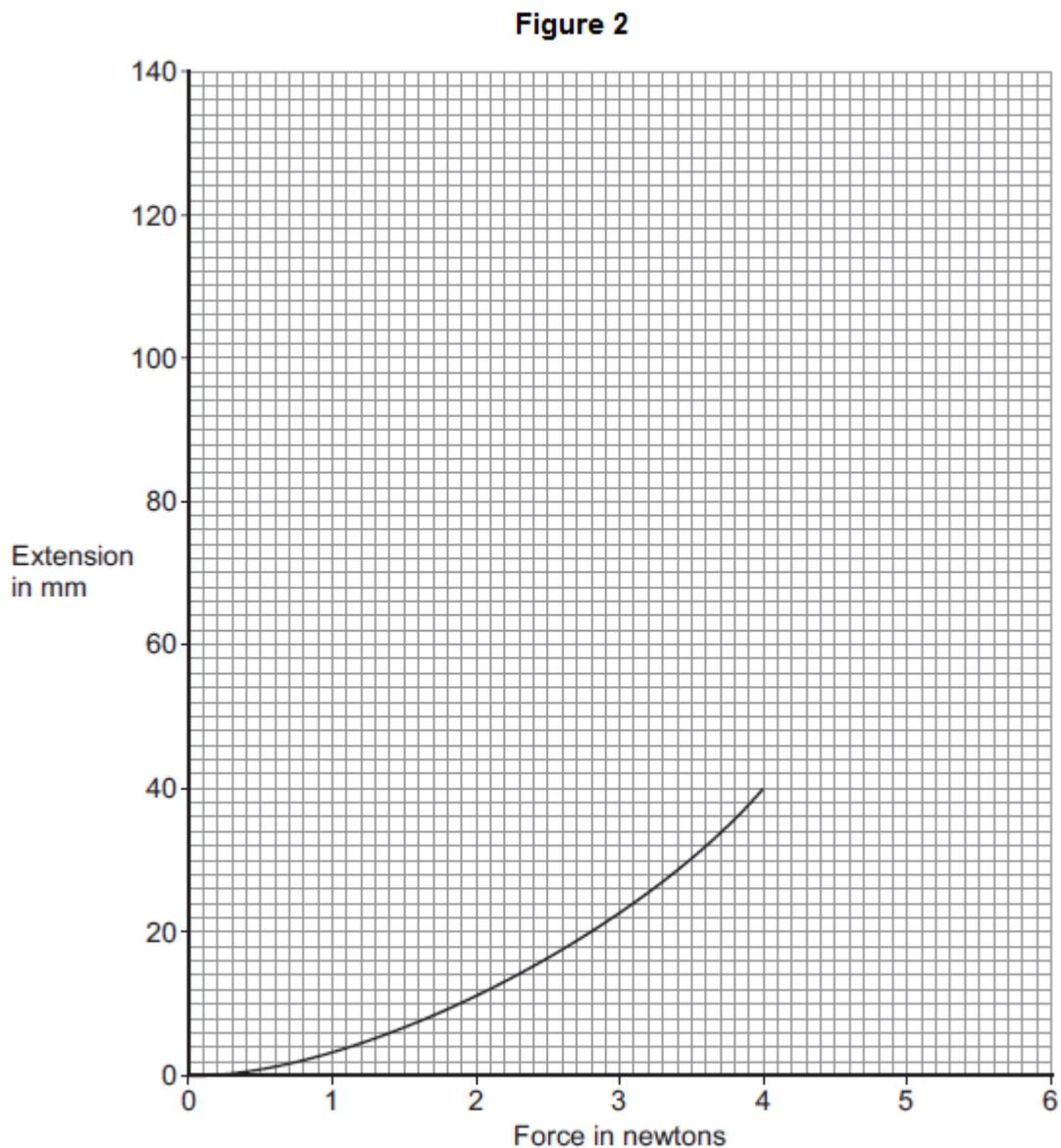
What can you conclude, from **Figure 2**, would happen to the extension of the rubber band if the force applied to the rubber band was increased to 6 N?
