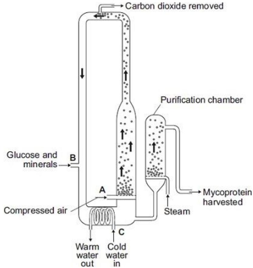
(a) Bubbles of air enter the fermenter at **A**.
